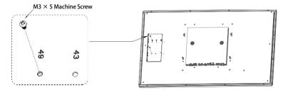
Step 5 Align the four hanging nail holes on the mounting plate with the four VESA screw centers on the back of the screen. Hang the screen securely onto the plate.
